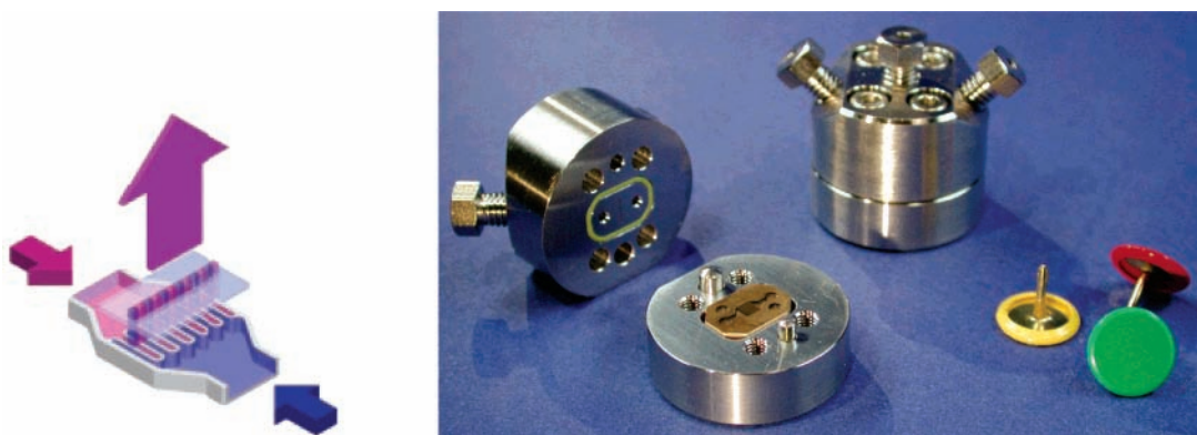
Figure 1. Mixing principle of slit-interdigital mixer (left) and image of the used device SIMM-V2 (right)
